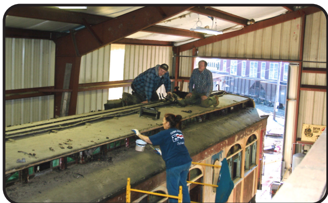
Then years of tar and paint were removed from the roof by scraping
