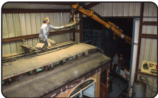
It was then decided to rebuild the entire car and remove modernizing items, first the trolley poles were removed from the roof
