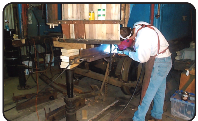
In 2004, 315 was taken into the shop to rebuild rotten frames on the ends of the car
