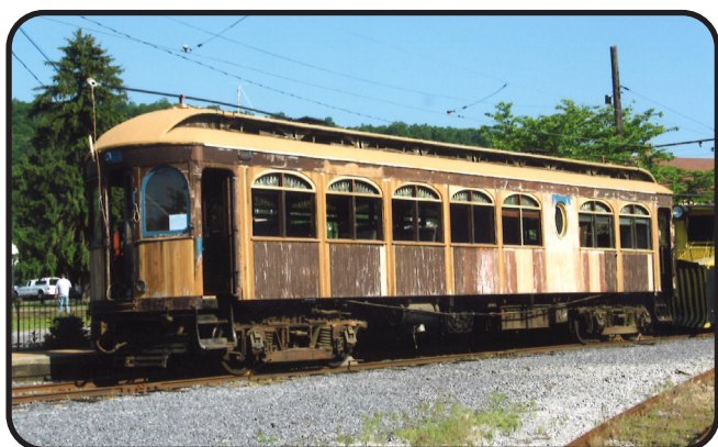
All the old paint was scraped from the car and new wood placed in rotten areas and modernizing removed
