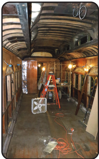
The inside was gutted and stripped of paint to reveal natural wood underneath
