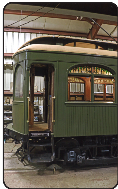
The original stained glass windows were re-installed after removing many layers of paint from them
